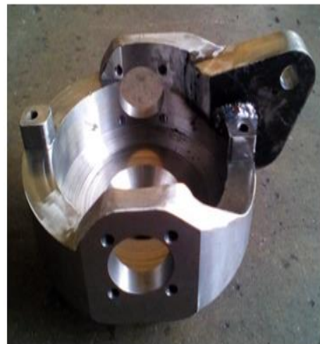
Fig. 13. New mechanical part produced with milling and welding
